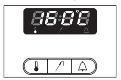
As soon as a heating system is selected, the **recommended temperature** for that system appears in the oven display and the oven heating comes on.
